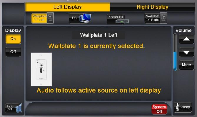
In this configuration the Left Display is active and available for source selection. The Display is ON and is highlighted yellow. The Left Wallplate is the active source. Information about the active source is displayed in the center.
