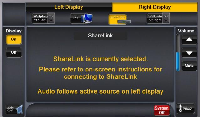
In this configuration the Right Display is active and available for source selection. The Display is ON and is highlighted yellow. The ShareLink is the active source. Information about the active source is displayed in the center. Audio in the room will still follow the Source (if any) going to the Left Display
